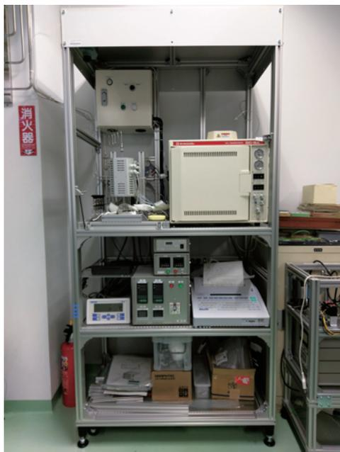
Fig. 1. Photograph of the catalytic activity analysis system (SMP-MR3F).
